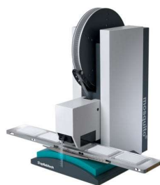
Mosquito liquid handling robot transfers reagents into correct wells on reaction plate
